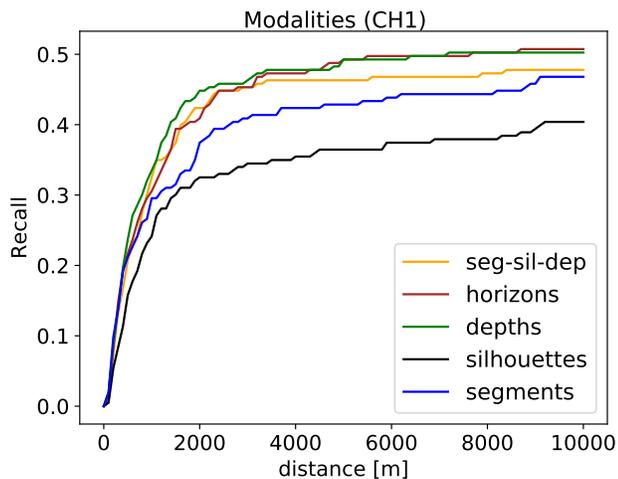
Figure 1. Localization performance of database image modalities. Results are measured on the combination of the CH1 dataset (used as queries) and the testing part of the *uniform database*.
