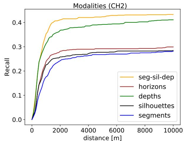
Figure 2. Localization performance of database image modalities. Results are measured on the combination of the CH2 dataset (used as queries) and the testing part of the *uniform database*.
