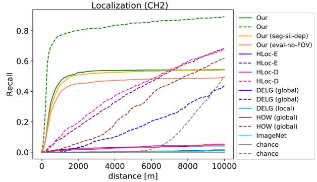
Figure 5. Localization performance of our approach and state-of-the-art methods evaluated on the combination of the CH2 dataset (used as queries) and the testing part of the *uniform database*. Solid lines: recall at 1 database candidates retrieved for each query, dashed lines: recall at 100 candidates.
